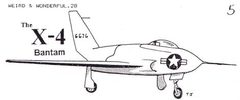
The Northrop X-4 was not designed to smash records for height and speed; its purpose was to test out the theory that a tailless aircraft would avoid the problems of interacting sonic shock waves between wing and tailplane. An unexpected bonus was the discovery that its large, split airbrakes allowed it to simulate the landing characteristics of various fighters.
